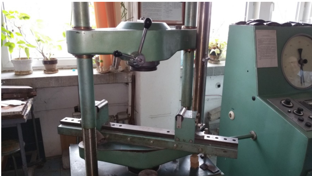
Fig. 1 Universal testing machine with hydraulic drive
